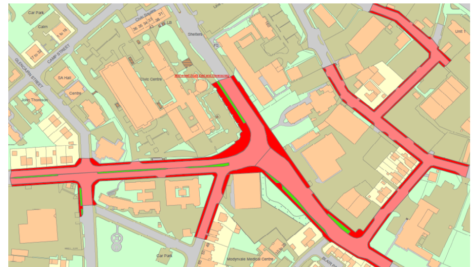
Figure 2: Extent of existing adopted carriageway, footway and verge
